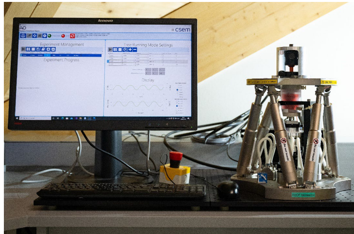
The movement and loading pattern of the multi-axial bioreactor is controlled by software.
